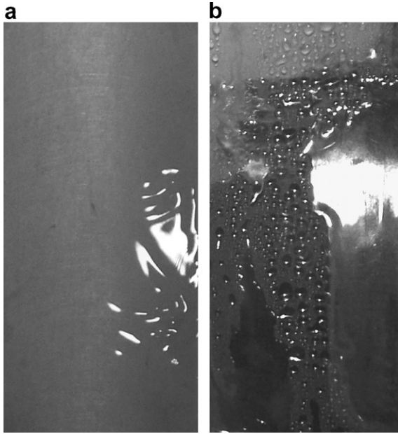
Fig. 10. FWC on unimplanted (a) and mixed DWC and FWC on implanted (b) polished Al 6951 plates.
